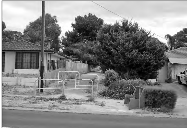
Figure 3: Pedestrian access way providing crucial pedestrian access from interior of a suburb with road layouts based on culs-de-sac to bus access on a perimeter road
